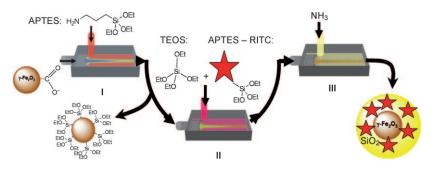
Coupled microreactors allow fast, continuous, multistep synthesis of the title compound. Thus, grafting with APTES is carried out in microreactor I, mixing with sol-gel TEOS and APTES labeled with
